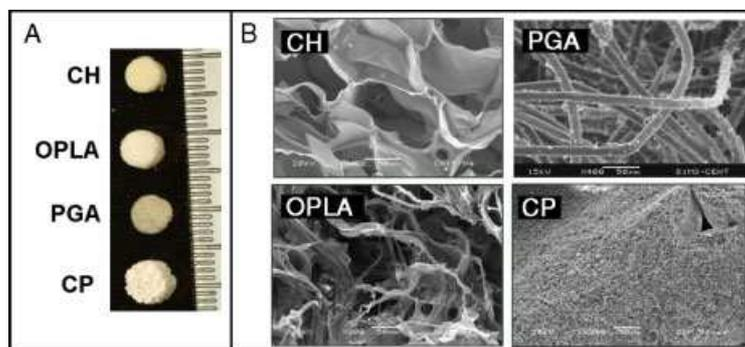
**Figure 1.** Macroscopic and SEM examination of chitosan–hyaluronic acid (CH), poly(lactic acid) (OPLA), polyglycolic acid (PGA) and tricalcium phosphate (CP) scaffolds. (A) Scaffolds placed next to a metric ruler. (B) SEM of scaffolds at  $\times 300$  (OPLA, CP) and  $\times 400$  (CH, PGA)
